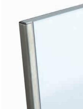
The flat signs in the Lite series consist of a stainless steel cassette with three edges, into which a 4 mm thick acrylic glass panel is inserted from above. This makes changing the inserts extremely easy. The panel is milled accordingly so that it is flush with the narrow stainless steel frame. It is mounted by screwing it through the screw eyes punched on the back, or it can be glued if desired. Suitable label inserts are offered in the last chapter "Label inserts and mounting material".
