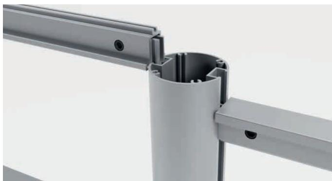
The MyWay wayfinding system is a high-quality and inexpensive system that can be used flexibly thanks to its modular design. The posts with 2 grooves and a diameter of 60 mm can either be directly encased in concrete or screwed to the ground with round plate feet ( $\varnothing$  200 mm). Plastic cover caps close the tubes from above.
